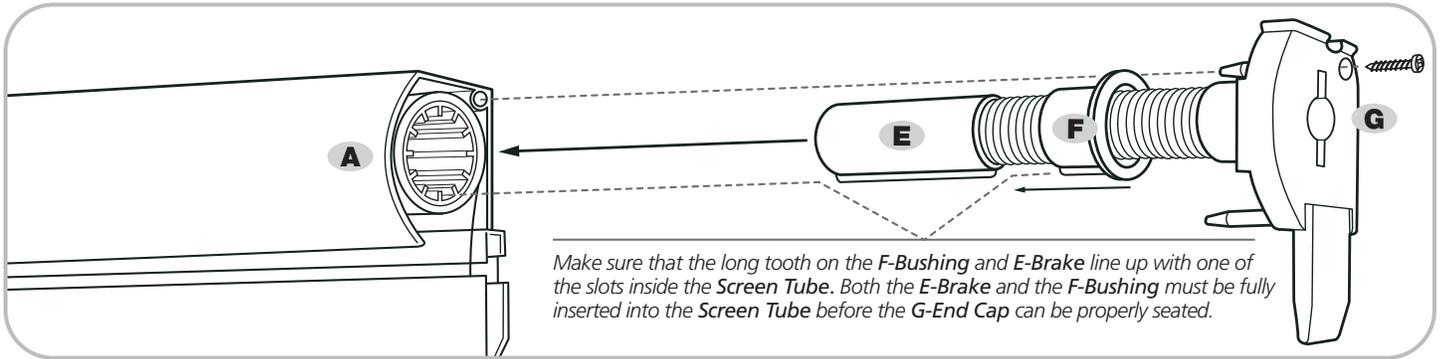
Slip the F-Bushing down the coiled spring to the E-Brake. On the open end of the A-Screen Cassette, insert the E-Brake with F-Bushing into the center of the Screen Tube, aligning the long tooth on both as noted above. Next, match up the large pin on the top of the G-End Cap to the corresponding hole at the top of the A-Screen Cassette Housing. Tap evenly with a soft mallet until the assembly fits snugly.
