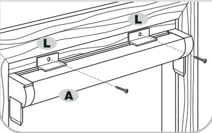
**NOTE:** It is critical that the Screen Cassette and Rails be installed square and plumb in the door opening. Apply shims (not supplied) as needed.
